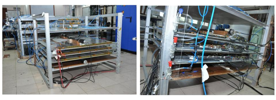
All detector are operated at 2mbar above atmospheric pressure with gas composition
