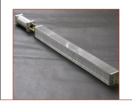
Dimensions $60x60 \text{ mm}^2$ Radiation length17 mmMoliere radius36 mmRadiation thickness25  $X_0$ Scintillator thickness1.5 mmLead thickness0.8 mmEnergy resolution1%
