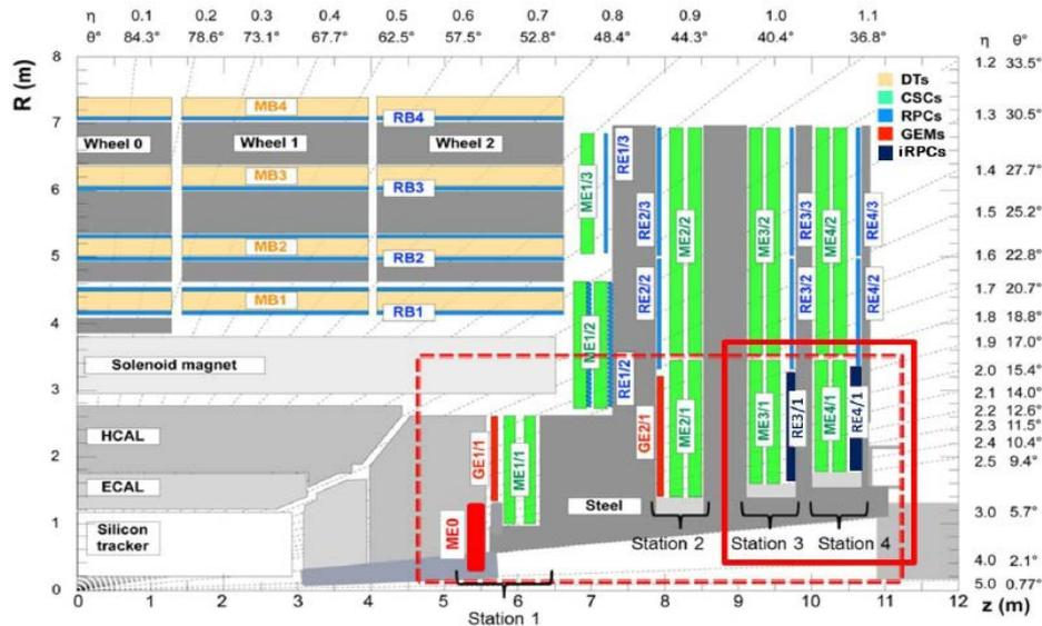
**In CMS muon system, the present design of the endcap RPCs, made of a double Bakelite gas gap and operating in avalanche mode, is not expected to be suitable for the particle rates amounting to several tens of kHz/cm<sup>2</sup> in the scenario of an LHC luminosity going up to 10<sup>34-35</sup> cm<sup>-2</sup>s<sup>-1</sup>**
