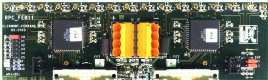
Since the beginning of LHC operations, MTR has been equipped with **ADULT** (**A DUaL Threshold**) front-end electronics:
