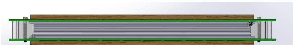
Self-sealed MRPC's side is **sealed by PMMA**, enables it **work independently**.
