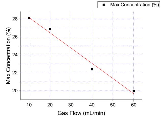
Max concentration **drops linearly** with gas velocity increasing.
