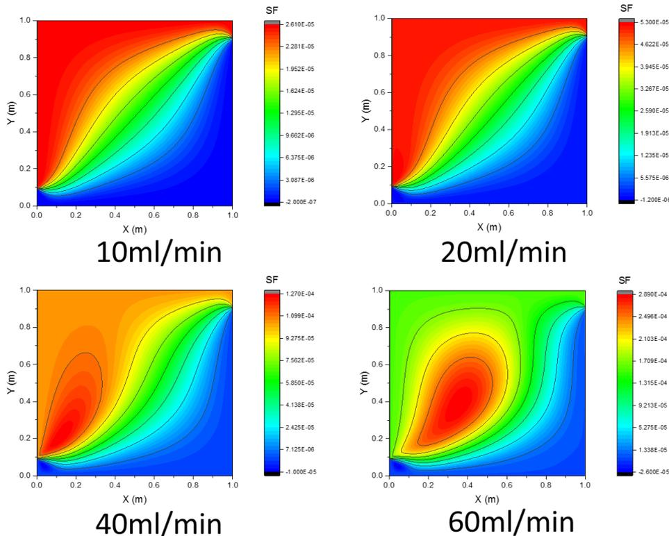
When the gas inlet velocity is relatively low, there is **no jet entrainment**. Gas flows directly from inlet to outlet.
