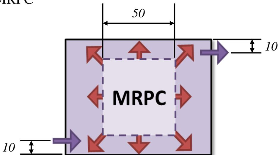
**Calculating field:** the horizontal transect of the gas box with MRPC inside at the level of a gas gap.
