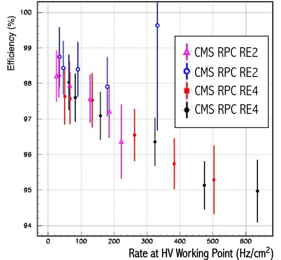
Eff<sub>max</sub> vs Rate for all RE2 and RE4 aging chambers during October Test Beam 2015
