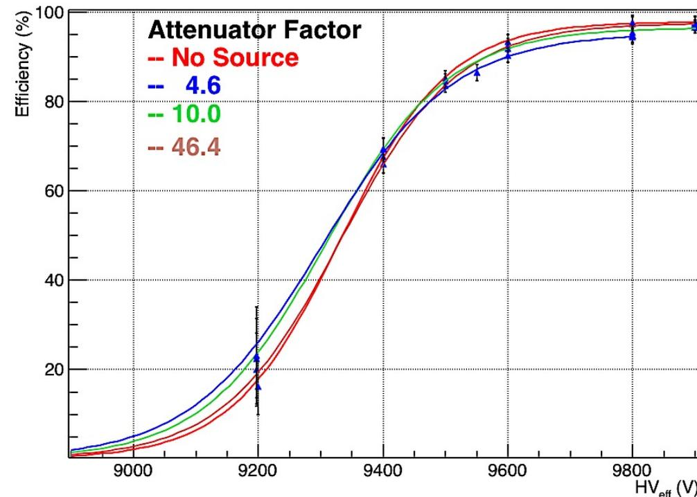
Example of Attenuator Scan in one RE2 during October Test Beam 2015
