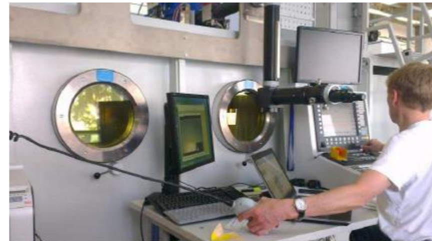
Made by Electron Beam Welding process In Vacuum, Welding deep of 5 mm.
