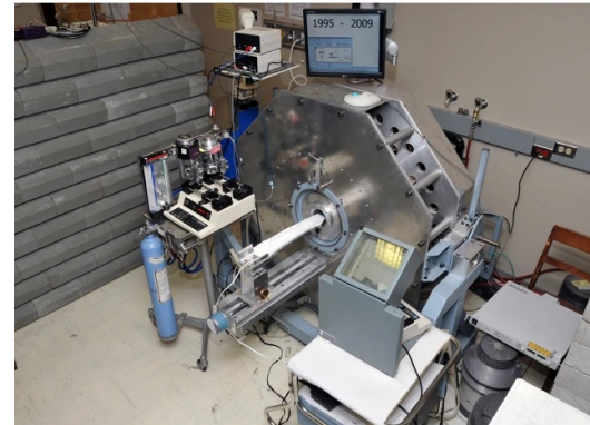
The Sherbrooke small animal PET, the first PET with APDs
