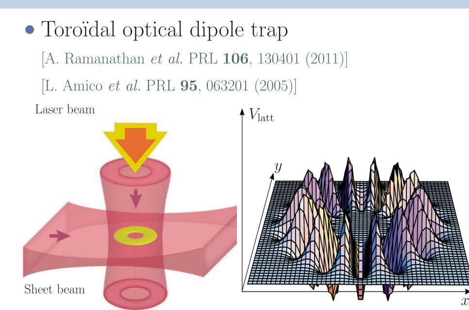
Intersection of two red-detuned beamsConnection to two waveguides
