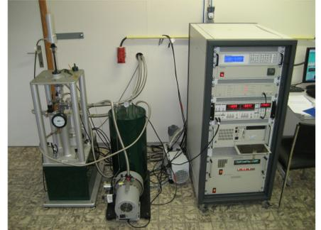
Photo of the Vibrating Sample Magnetometer (VSM)
