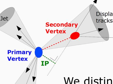
Hadronic particles undergo a fragmentation process and create **particle showers ('jets')** inside the CMS detector.
