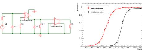
Figure 5: Block diagram of ATLAS amplifier. R1: impedance resistance (left). Efficiency plateaus for standard CMS RPC FEE and new ATLAS prototype electronics (right). A shift of  $\sim 460 \text{ V}$  is observed corresponding to a decrease of charge deposition from 20 pC to 3 pC.
