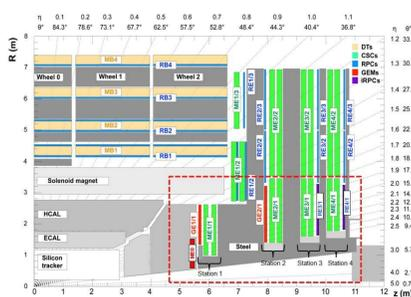
Figure 3: Quadrant of the muon system showing DT chambers (yellow), RPC (light blue), and CSC (green). Phase-II forward muon detectors are contained within the dashed box: in red for GEM stations and dark blue for improved RPC (iRPC) stations.
