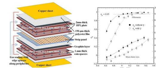
Figure 6: Schematics of a RPC with electrodes made of low resistive silicate glass or float glass together with the efficiency vs rate for different RPCs [5] (top). 6-gap RPC together with time resolution as a function of HV (incoming  $\mu$ -rate of  $1.2 \text{ kHz/cm}^2$ ) [6] (center). Multigap HPL RPC prototype together with efficiency plateau and cluster size as function of HV w/ (open symbols) and w/o (solid symbols) a  $3 \text{ kHz/cm}^2$   $\gamma$ -irradiation [4] (bottom).
