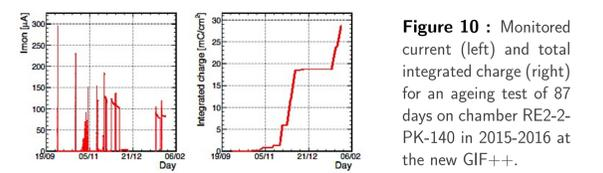
Figure 10: Monitored current (left) and total integrated charge (right) for an ageing test of 87 days on chamber RE2-2-PK-140 in 2015-2016 at the new GIF++.
