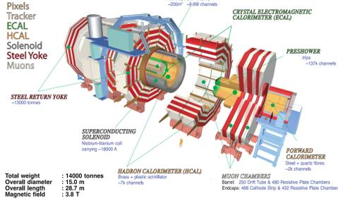
Figure 1: Exploded view of the CMS detector.
