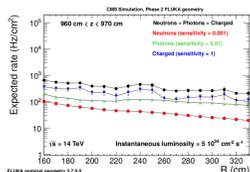
Figure 4: Simulated particle hit rate as a function of radius at the RE3/1 station (0.001 sensitivity to  $\mu$ , 0.01 to  $\gamma$  & 1 to ionizing particles).
