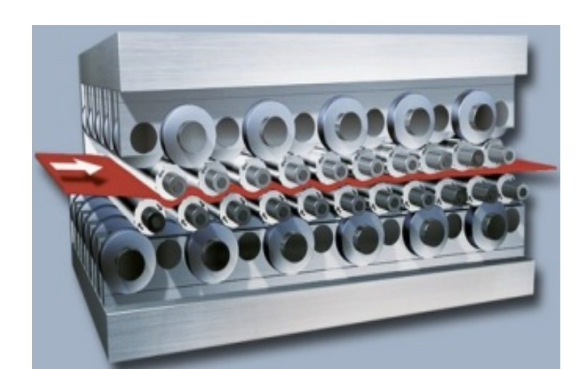
Fig 15: Roller levelling technique.
