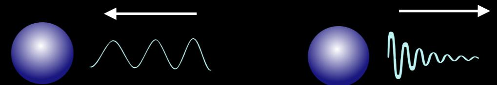
$$h_+ - ih_\times = -\frac{M}{r} \sum_{lmn} \mathcal{A}_{lmn} S(\theta, \phi) e^{i\tilde{\omega}_{lmn} t}$$
